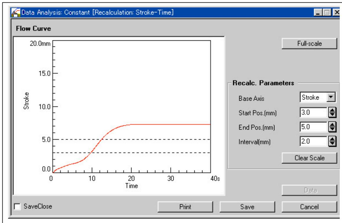
Figure 2: Epoxy flow curve at 165°F using Shimadzu Capillary Rheometer CFD-500D
