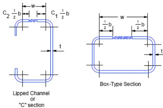
Figure 9 Closed Sections for Stiffening
