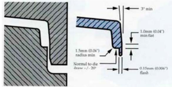
Figure 2, Typical SMC Compression Mold, Shear Edge
