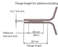
Figure 13.47: Joint and flange required for adhesive bonding
