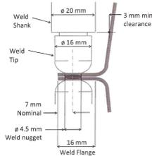
Figure 13.34: Resistance spot weld flange requirements
