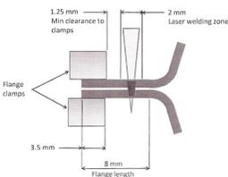
Figure 13.39: Weld flange requirements for laser welding
