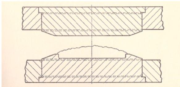
**Figure 1, Typical Flash Type Compression Mold**
